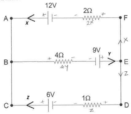
Three unknown currents: x, y, and z are identified in the above circuit.
